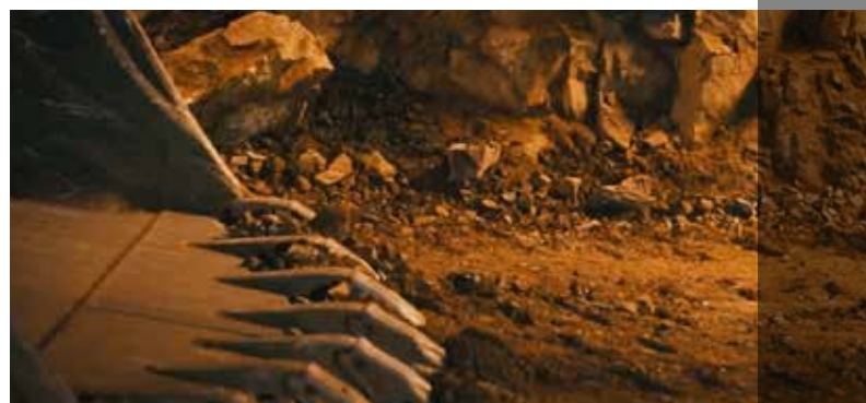
Figure 3. The scoop of a remote-controlled LHD underground at Pucobre.
